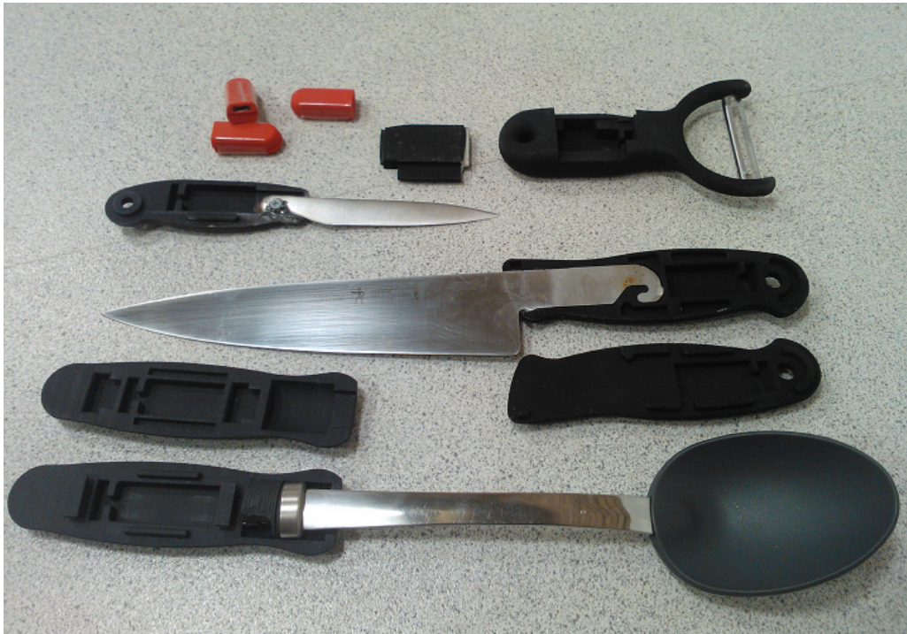
Figure 6.2: Wireless accelerometers (top left) were embedded into the modified handles of kitchen utensils.
