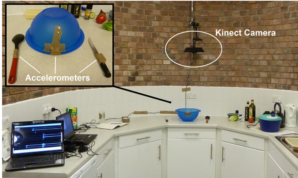
Figure 6.6: Accelerometer Localization: slightly modified experimental setup. Laboratory kitchenette with Kinect facing the work surface and accelerometers attached to three kitchen utensils with tape (top left).
