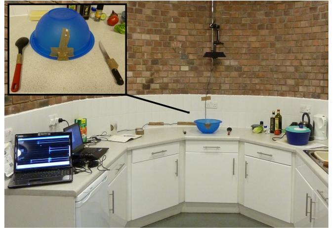
Fig. 3. Experimental Setup: Laboratory kitchenette with Kinect facing the work surface and accelerometers attached to utensils with tape (top left).
